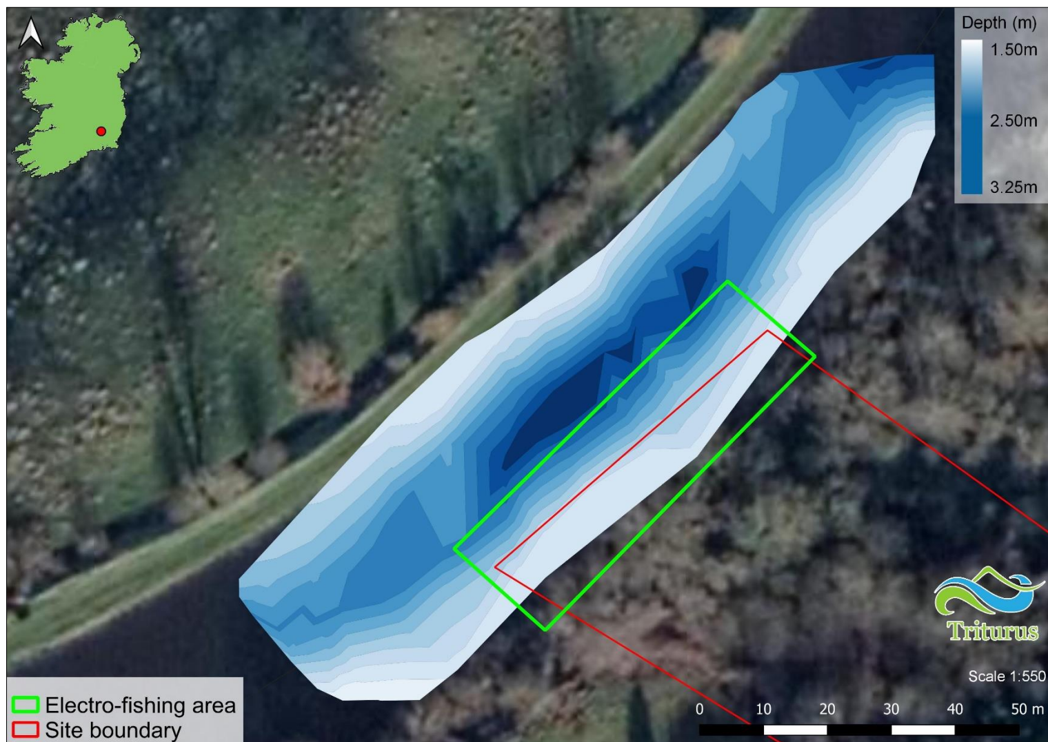
Figure 3.3 Bathymetry map of the proposed Mortarstown WWTP outfall works area, (darker shading indicates deeper water) Triturus data (2021)
