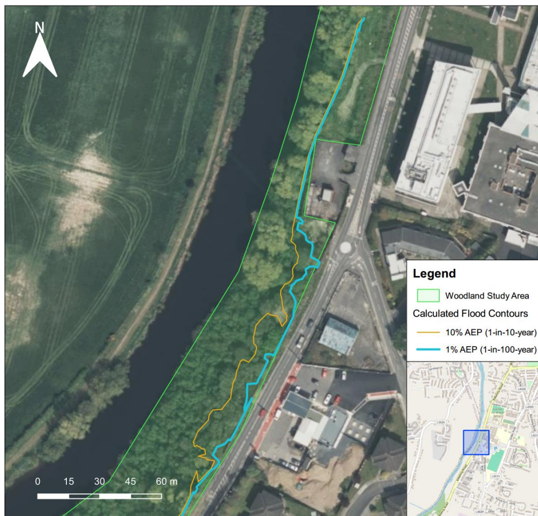
Figure 5: Calculated flooding contours for the northern part of the study area.
