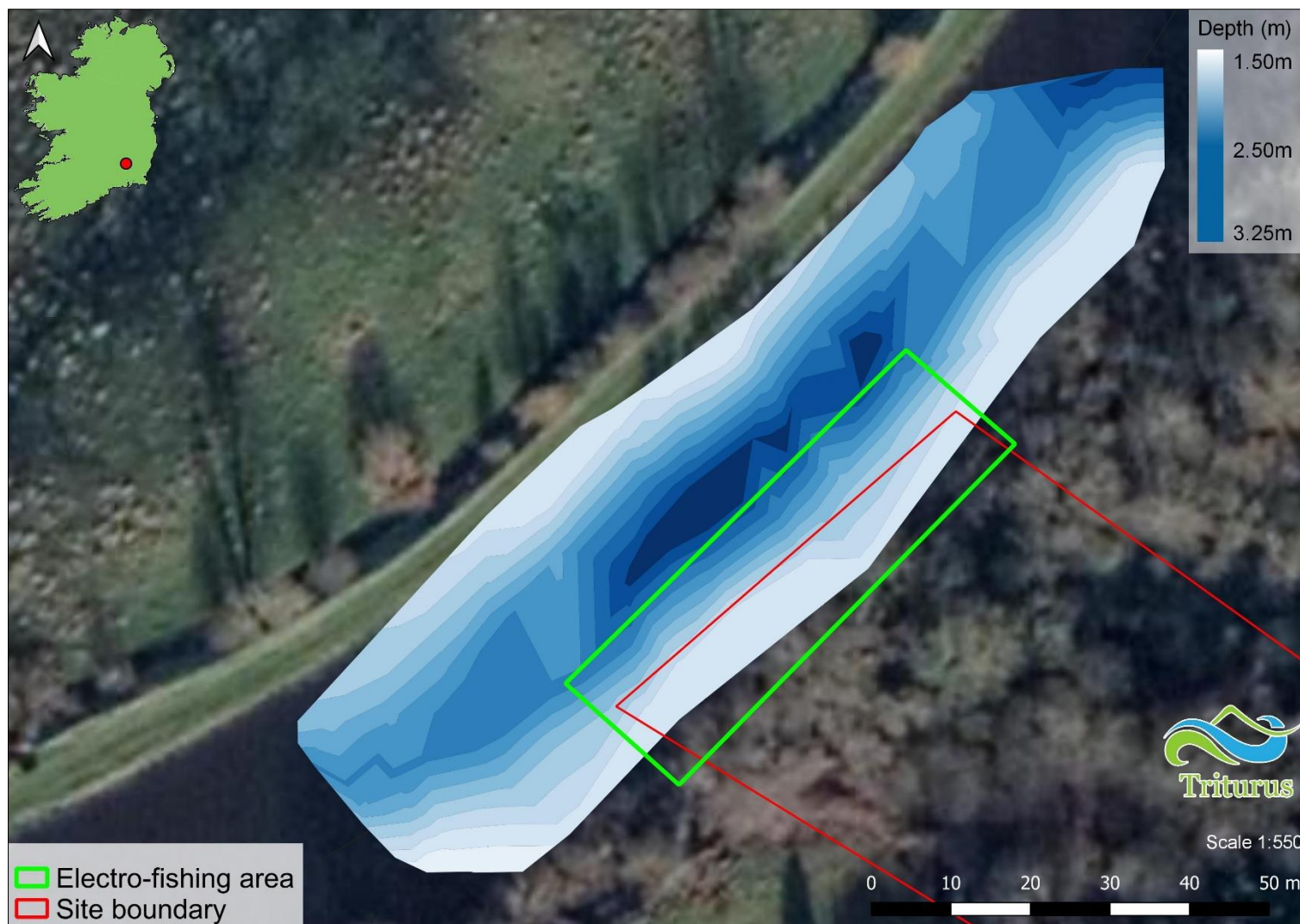
Figure 3.3 Bathymetry map of the proposed Mortarstown WWTP outfall works area, July 2021 (darker shading indicates deeper water)
