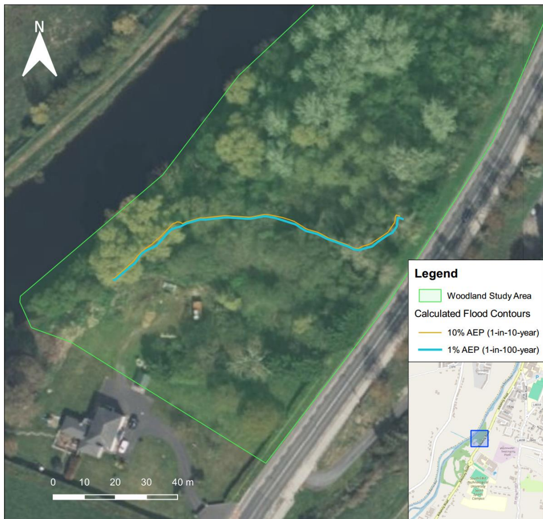
Figure 6: Calculated flooding contours for the southern part of the study area.
